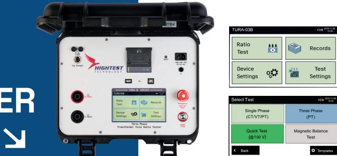
TURA-03 is designed to accurately measure the turns ratio of single-phase and three-phase transformers.
